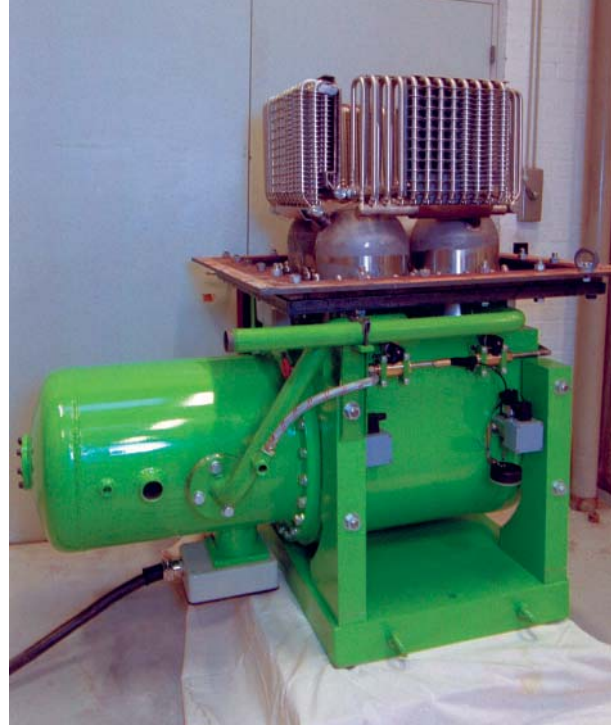
Stirling engine ready for installation in a wood chips combustion system
