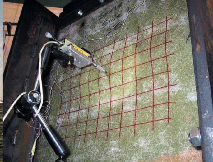
Left: A Standard Flex 300 of the FLYVEFISKEN class. Right: Bottom panel with circular debond, failed in pure compression and tested in the strength laboratory at DTU
