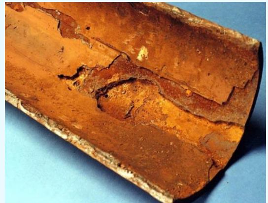
Internal corrosion in a crude oil pipeline
