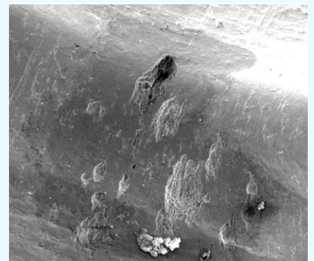
ECG electrode showing local corrosion and stress corrosion cracking after exposure to chloride environment
