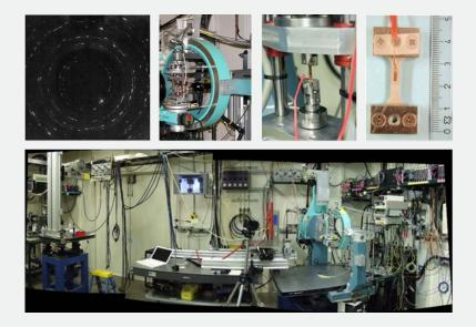
Aim of the project is to analyze and quantify the microstructural changes occurring during fatigue of fcc metals. Preliminary data on copper have been taken already during 80.000 loading unloading cycles. Revealing the microstructure evolution by tracing individual subgrains during cyclic loading from the maps will shed light on their formation mechanism and further the insight in the initiation of failure.
