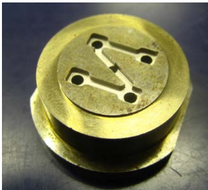
Micro injection moulding: two-cavity micro tool (left), micro dog bone part (center) and meshed model (right). Polymer product: polyoxymethylene BASF Ultraform H2320 004, part volume = 75 mm 3 , mass = 91.3±0.3 mg. Modelled part: 1000000 3D elements, 100 µm mesh size.
