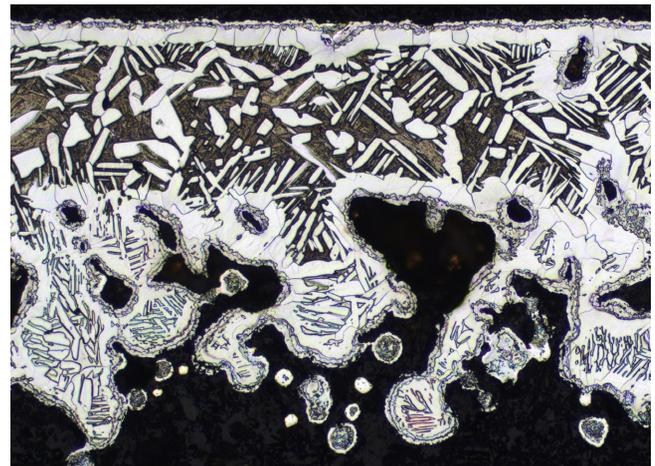
New methods for surface hardening titanium can solve the problem with wear resistance for the material and open up for a wide range of new applications. Left: A microscope image of a cross section of a pulley wheel before hardening. Right: The same cross section after the new hardening process, in this case the surface hardness has increased 5 times. Images from Emilie H. Valente's MSc project.
