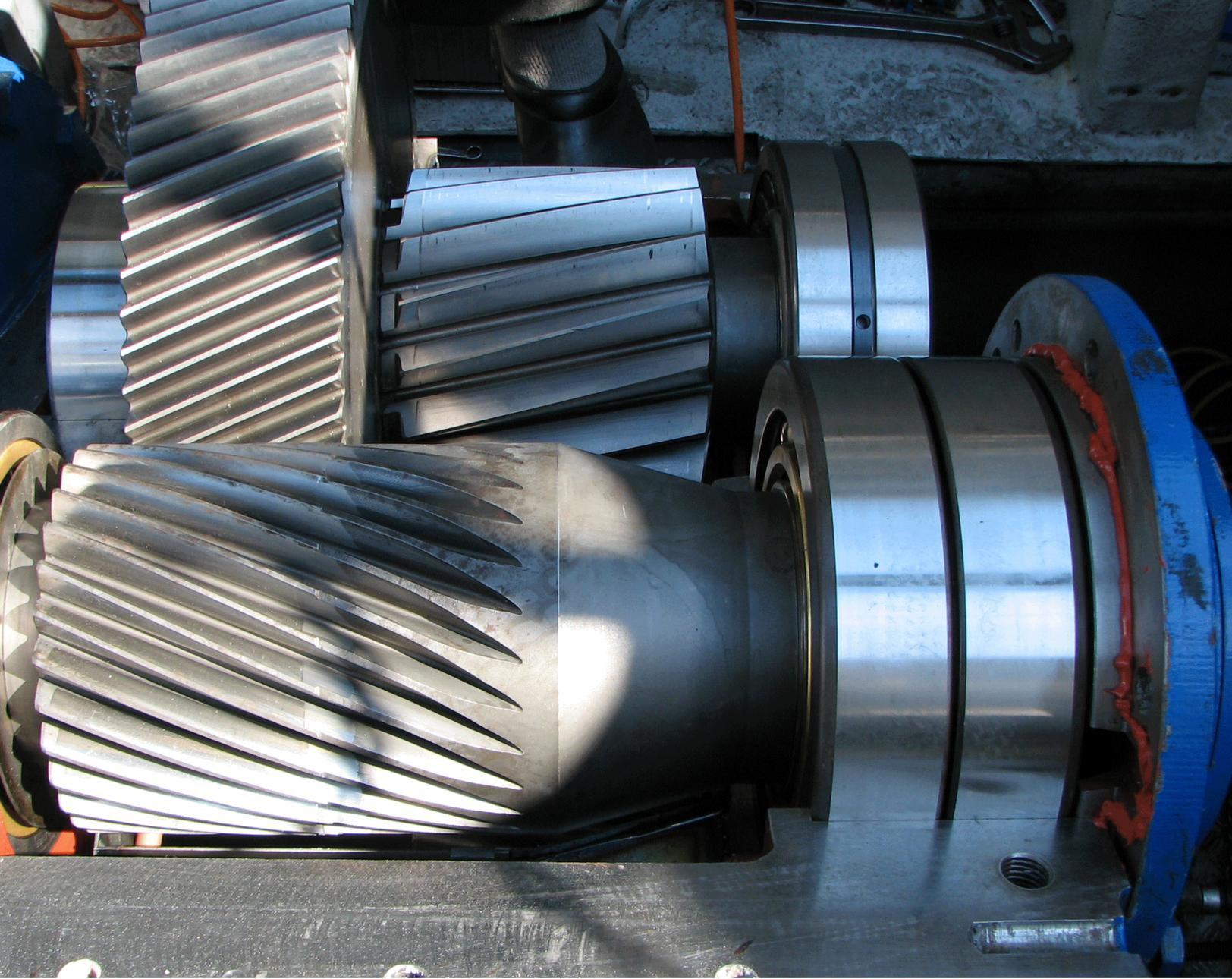
*The photo shows the placement of the bearings and gears inside the nacelle of the wind turbine. Photo: Mogens Hvid*
