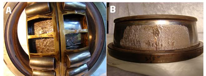
*The photos show typical failure and damage of bearings which can be induced by so-called white etching. White etching cracks start below the surface and eventually leads to severe damage. The specific occurrence of the damage is difficult to predict, and the cracks may cause a complete breakdown of the wind turbine.*
