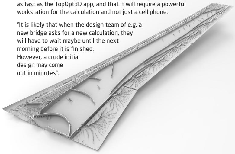
Aerial view of the optimized load carrying structure of a Boeing 777 wing.
